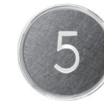
A81 White/A82 Orange Φ36.5mm, mechanical inching, Flat characters, Glimmering on standby, Stainless steel surface.
